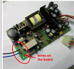
For older RME devices that require soldering, you will need to first disconnect the two wires connecting the Power-Supply-Unit to the mainboard.
