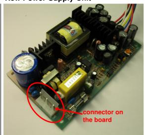
Newer RME devices will have a connector installed on the PSU.
